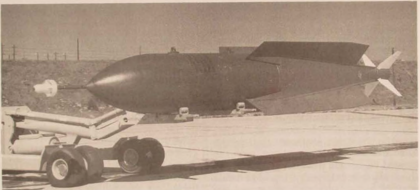
The USAF pushed the laser-guided bombs. The laser kit could be fairly easily adapted to other bombs, and it was. By 1971, five-hundred-, one-thousand-, two-thousand-, and three-thousand-pound bombs were being used. Above: Two Mk 82 five-hundred-pound bombs with laser kits on an F-4C. Below: A three-thousand-pound LGB.
